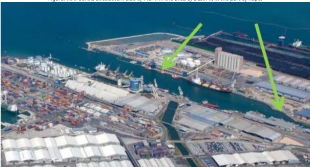
As mentioned in previous paragraphs, the next step will be the construction of all the berthing capacities around Basin II. On side there're the berths 7F and 7G at the northern side of Pier I, where an additional Post-Panamax and New Panamax vessel can be berthed. On the other side of Basin II, there're new berths being (re)constructed for the berthing of petrol tankers, general cargo vessels and Ro-Ro ships.
