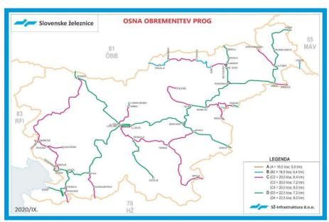
Figure 18 Line categories according to axle load [Source: gov.si/teme/zelezniska-infrastruktura]
